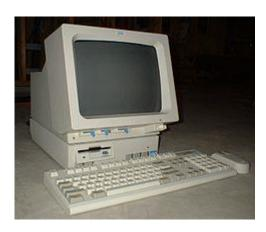
Operating system PC DOS 4.01 CPU Intel 80386SX @ 16 MHz Memory 2 MB ~ 6 MB
