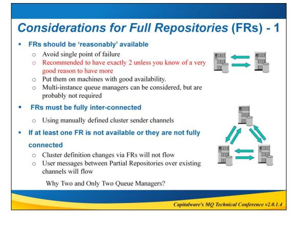
Full Repositories must be fully connected with each other using manually defined cluster sender channels.
