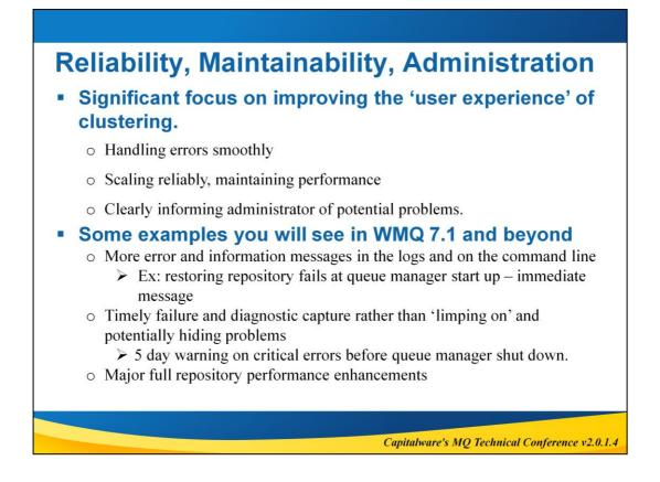
One of the big shifts to note here is from allowing the queue manager to continue without a running repository manager. When the repos manager encounters a critical error it will now go into 'retry' for a few days, issuing warnings with a countdown timer, before shutting down the
