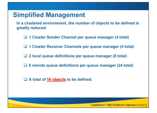
In a clustered environment, the number of objects to be defined is reduced to 16. This is due to the fact that the only one cluster sender and cluster receiver channel is needed, and no transmission queues or remote queue definitions are necessary.
